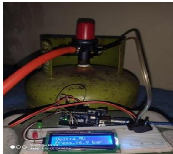
Figure 5. The sensor receives a voltage of 4.5 volt and a pressure of 7 bar
