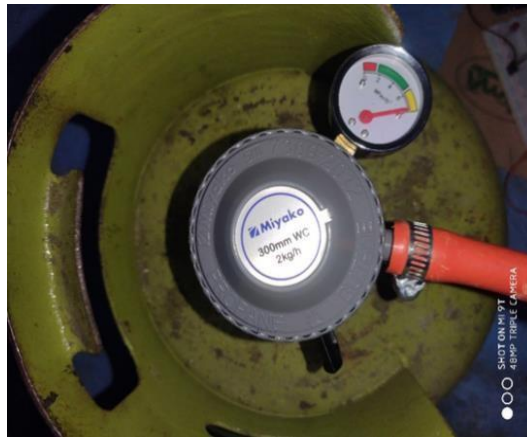
Figure 9. Second regulator with valve condition after locking
