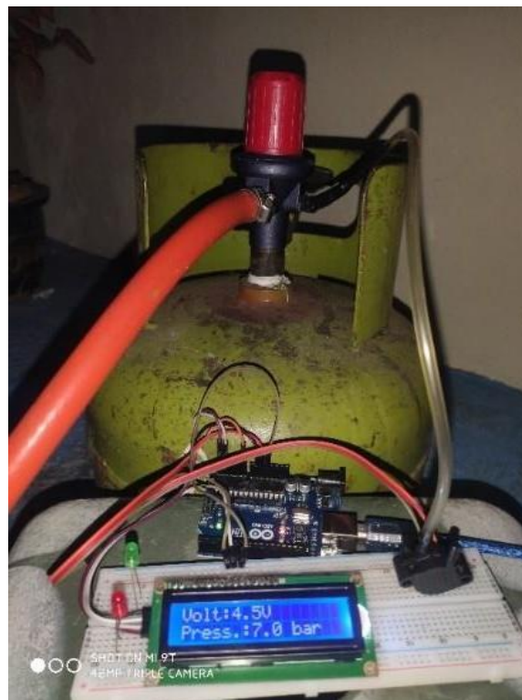
Figure 10. Testing lcd 16x2
