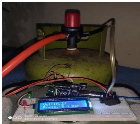
Figure 4. The sensor receives a voltage of 0.2 volt and a pressure of 0.3 bar
