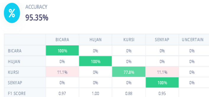
Figure 9. Confusion Matrix Model testing
